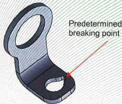
Figure 10: Anchor point, type: TS-lug (TS-106_V20) (with predetermined breaking point, no chamfer)
