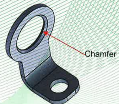
Figure 11: Anchor point, type: TS-lug (TS-011) (no predetermined breaking point, with chamfer (2 x 45°))
