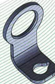
Figure 5: Anchor point, type: TS-lug (TS-011) (with predetermined breaking point, with chamfer (1 x 45°))
