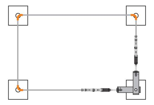
For all-round cable systems, the impact absorbers are to be mounted on a corner/start point with angle for impact absorbers. The FSA impact absorbers, FSA I impact absorbers, FSA I impact absorbers with absorbers and force absorbers are compatible with each other and can also be used mixed together without any problems.
