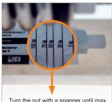
Turn the nut with a spanner until max. 30 kg are set or until the stainless steel cable has sufficient slack so that there is enough reserve for later temperature-related shortening of the metal cable at cold outdoor temperatures!
