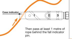
Pass the rope through hole 1 and hole 2, leaving at least 10 cm long loops as a reserve to allow accurate tensioning.
