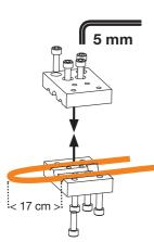
Tighten the fixing screws of the aluminium clamps with an Allen key to a torque of at least 15 NM.
