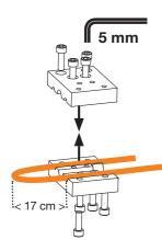
Tighten the fixing screws of the aluminium clamps with an Allen key to a torque of at least 15 NM.
