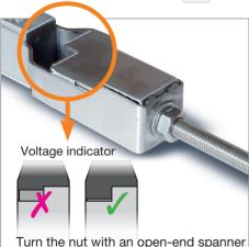
until the tension indicator is level or the stainless steel cable has sufficient slack so that there is enough reserve for later temperature- related shortening of the metal cable at outdoor cold temperatures!
