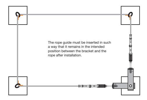
For all-round cable systems, the impact absorbers are to be mounted on a corner/start point with an angle for impact absorbers.
